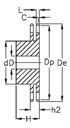
$\begin{array}{ccc} C & = 2 \\ d & = 100 \\ D & = 20\pm0,5 \\ De & = 141.8 \end{array}$
